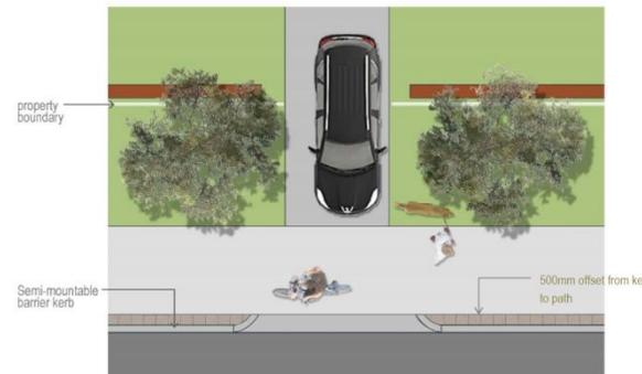
Figure 7 Plan View of Model Crossover Design
