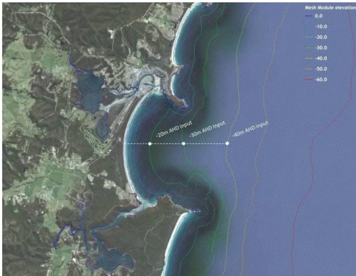
Figure 1. Three ocean outfall depths modelled by AECOM (2010)
