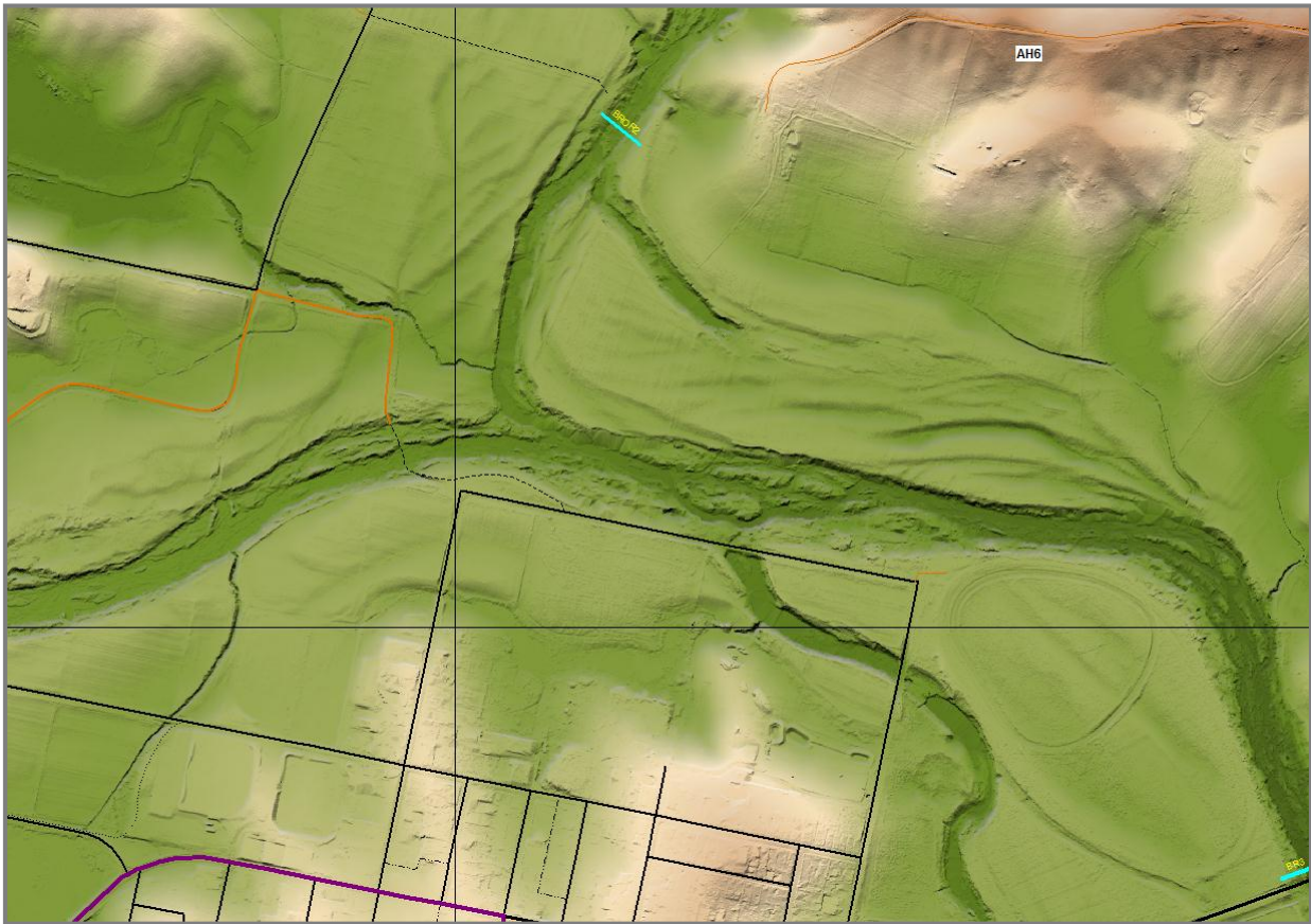
Figure 6.3: DTM Representation of the Confluence of Brogo and Bega Rivers North of Bega Based on the Council's LIDAR Survey Data
