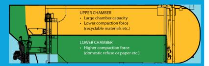
There might be some confusion as to why one truck collects both waste and recycling. Rest assured, your hard work separating is not being wasted! The trucks are specifically designed to hold waste and recycling separately so they can be sorted individually.
