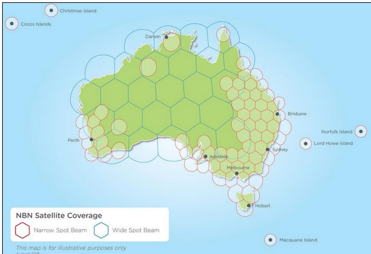
Figure 8-1 Diagrammatic Sky Muster spot beam coverage (Source: NBN Co)
